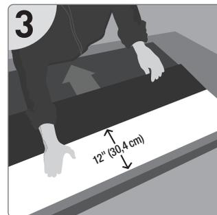
**3** Using clean hands, hold onto the white film while removing 12" (30,4 cm) of the textured liner from the top edge. **Note: DO NOT REMOVE THE ENTIRE LINER AT THIS POINT.**
