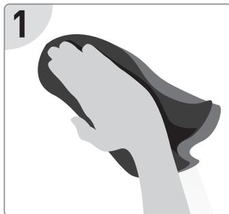
**1** Surfaces to be covered must be clean, smooth, dry and structurally sound. Thoroughly clean wall surface with a damp cloth. Let surface dry for 10 minutes before moving onto installation.
