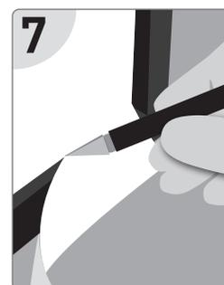
**7** If applying to an existing whiteboard or chalkboard, use the existing frame as a guide to trim excess film with a utility knife.
