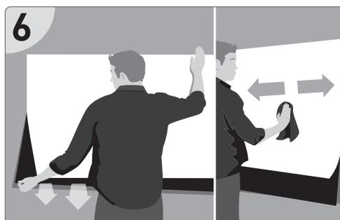
**6** Continue to install by removing 12" (30,4 cm) of liner at a time. Push firmly against the film moving any bubbles out to the left and right edges. Repeat peeling 12" (30,4 cm) of line and smooth out film from middle to edge until it is completely secured to the wall.
