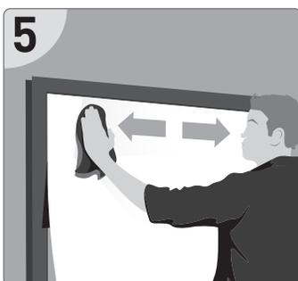
**5** Recheck alignment and adjust if necessary. Use the cloth to press film to the wall. **Always start by pressing from the middle and smoothing the film out to the edges.**
